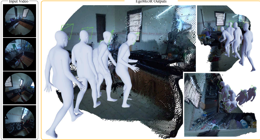
Figure 1: Given an egocentric video, EgoMo3R optimizes for camera poses , 3D pointmaps, and human motion in a common gravity-aligned metric reference frame. We also show two additional views of our scene and motion reconstruction on the side.
